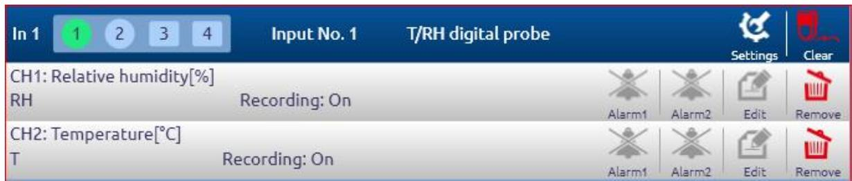
In the line of each measured variable (ie. channel), you can change its other settings (eg. Alarm limits, alarms indication, the channel recording, etc.). For these settings, use Alarm1, Alarm 2 and Edit icon.
